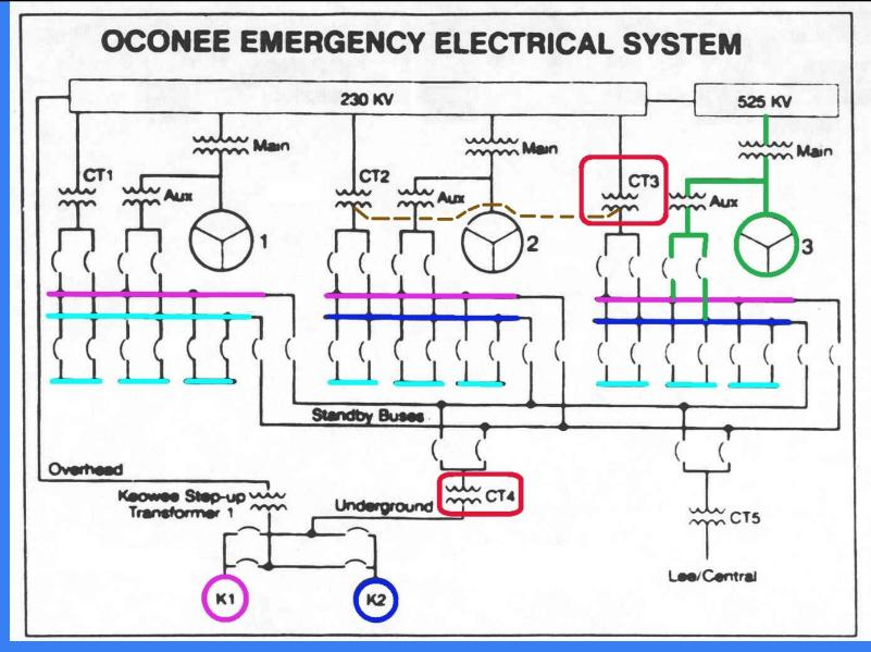
Oconee is the only U.S. nuclear plant without emergency diesel generators. Instead, its emergency backup power sources are the two hydroelectic units at the nearby Keowee Dam. A phase connection to transformer CT3 was found broken as workers were about to disable transformer CT4 for maintenance. A week later, a broken connection on transformer CT1 was found.
